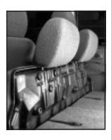
Secure the two black straps attached to the back of the folded seat cushion by hooking them onto the knobs on the back of the seatback when folded down. To raise the rear seat do the following:
